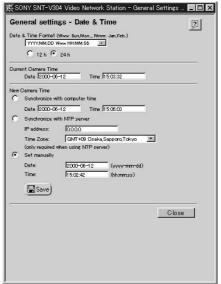
The setting items are shown in the following table. When finished setting, click the "Save" Icon. The accuracy of the internal clock is  $\pm 120$  seconds/month or less.
